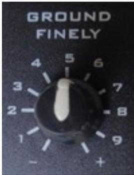
***The GROUND FINELY potentiometer serves as a further fine (precise) setting of the ground balance in a manual ground balance working mode, ie for a fine and complete eliminate of the ground effect at work in a manual ground balance working mode.***
