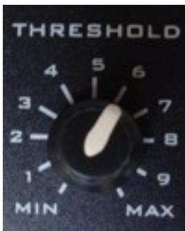
***The THRESHOLD potentiometer serves to define the desired from the user audio threshold and sensitivity of the metal detector.***
