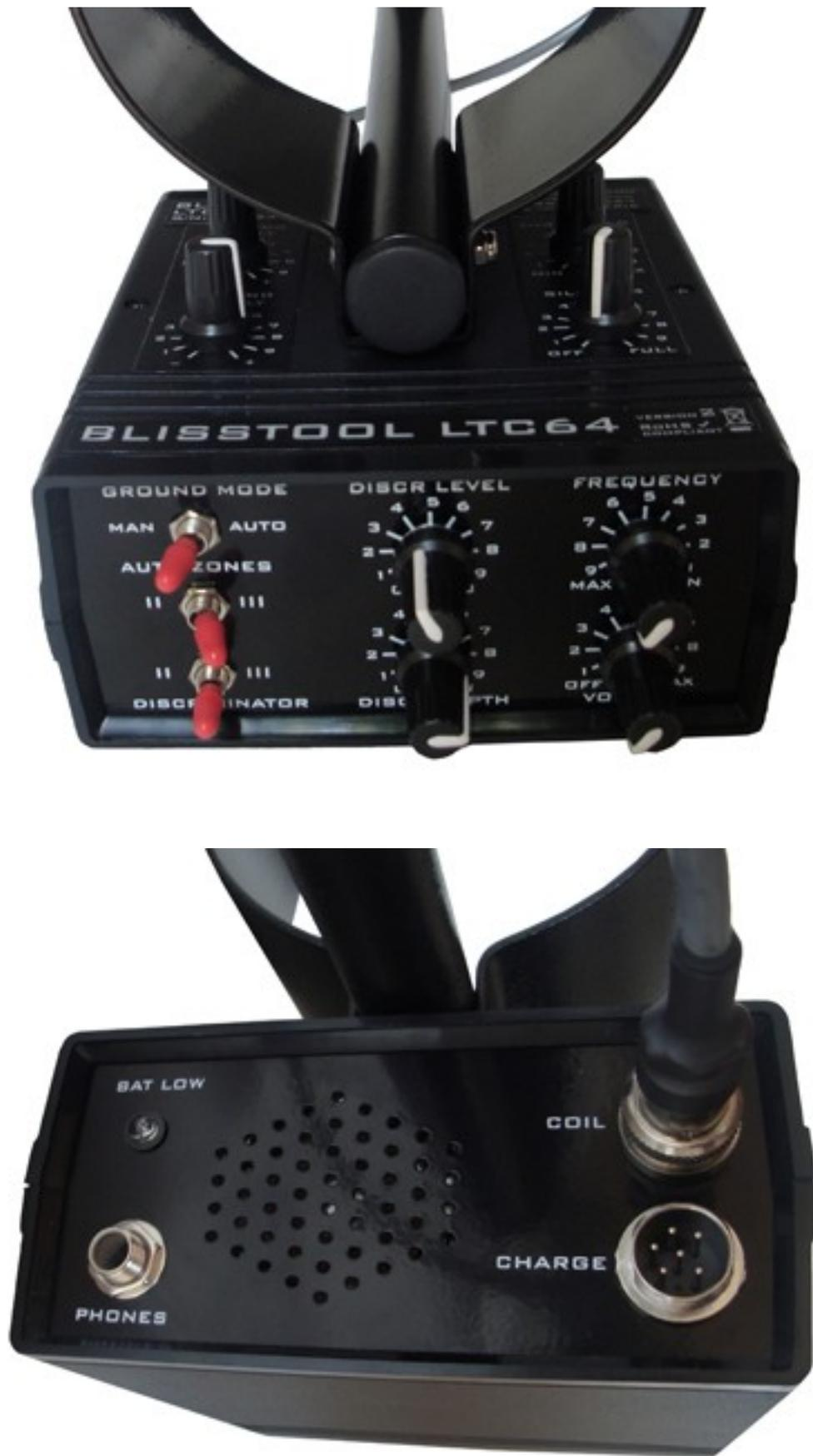
Fig.3 / Setting, indication and maintenance bodies of BLISSTOOL LTC64
