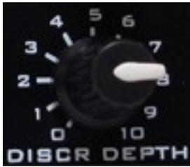
The DISCR DEPTH potentiometer serves for adjusting of a specific depth of discrimination. This is the maximum depth to which the metal detector distinguish the metals, ie the depth to which the metal detector rejects respective ferrous metals and pollutants.
