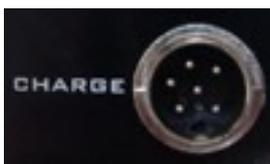
*The CHARGE connector serves for connection of the automatic LiPo battery charger to the built-in LiPo battery of the metal detector. The connection is carried by cable adapter, available in the standard package of BLISSTOOL LTC64.*
