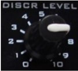
*The DISCR LEVEL potentiometer serves for adjusting the detection/rejection level of iron, tin-foil and low-grade non-ferrous metals (usually pollutants), and for baseline exclusion of the discrimination (All metals mode) when it is set to level „0“.*
