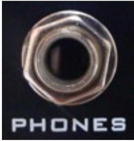
*The PHONES connector serves for plug to metal detector, if necessary, stereo headphones with 6.35mm (1/4") stereo jack. When the headphones are plugged in, the loudspeaker is switched off automatically and the metal detector's sound is heard only in the headphones.*
