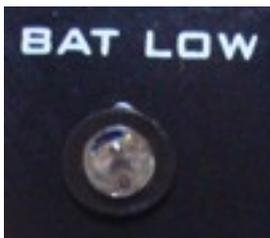
*The BAT LOW LED shows the available charge in the LiPo battery. When this LED lights up, it is a signal for low battery.*
