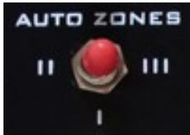
The AUTO ZONES switch serves to set one of the three available automatic ground zones at work in automatic ground balance working mode.
