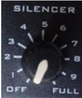
**The SILENCER potentiometer serves for setting of the degree of suppression of the background sound.**
