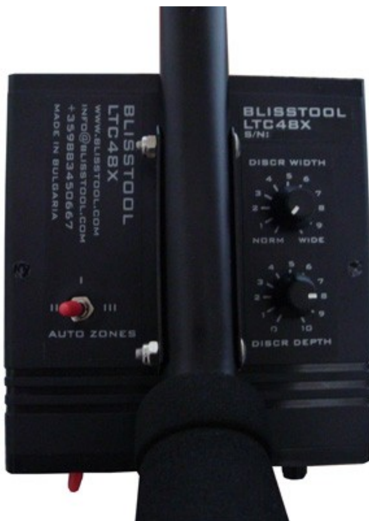
Fig. 3 / Control, adjustment and indication appliances of BLISSTOOL LTC48X
