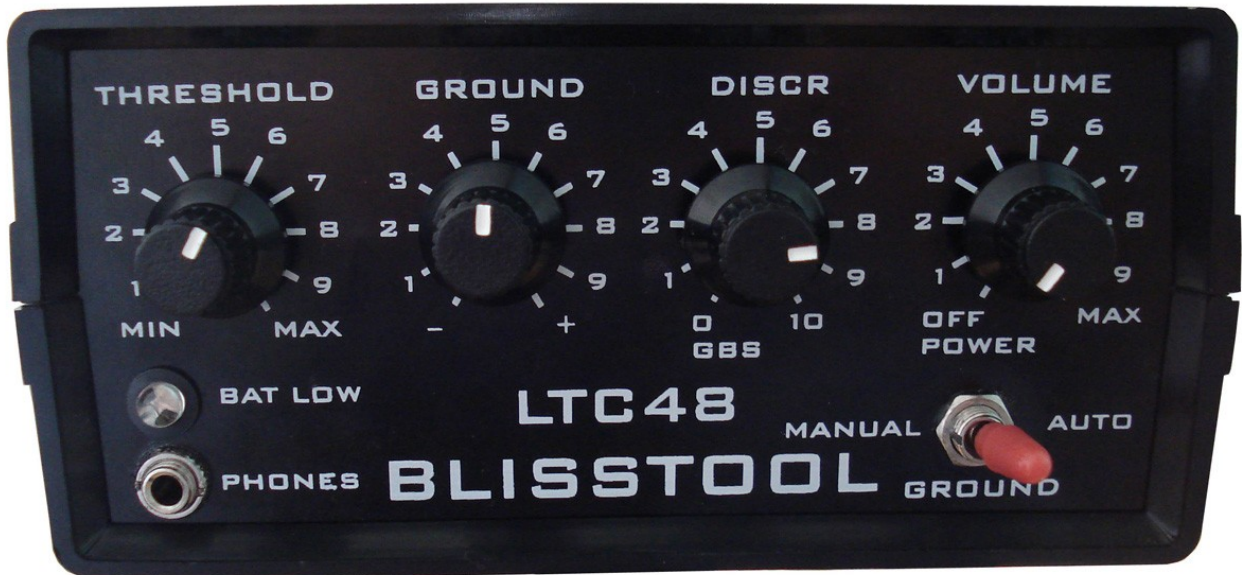
Fig.3 / Control, adjustment and indication appliances of BLISSTOOL LTC48
