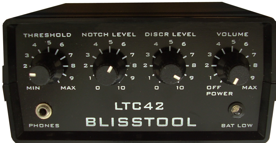
Fig.3 / Control, adjustment and indication appliances of BLISSTOOL LTC42
